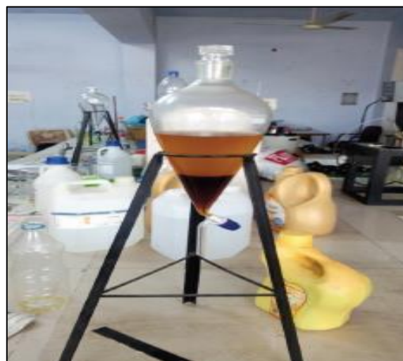
Figure 2: Product Allowed to Settle Down
