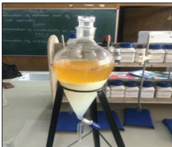
Figure 3: Formation of Ester Phase and Glycerol
