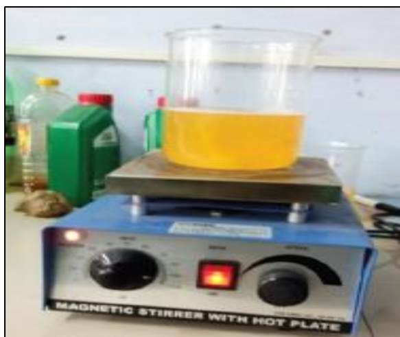
Figure 4: Heating of Biodiesel
